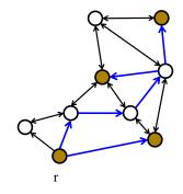
For  $S \subset V$ , where  $r \in S$  and  $(V \setminus S) \cap T \neq \emptyset$ : at least one arc in cut-set  $\delta(S, V \setminus S)$  must be used at a feasible solution
