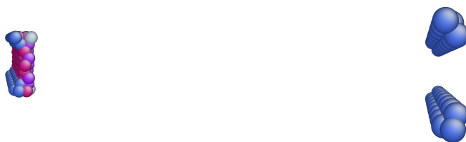
Figure 15: Atomic configuration of state C. Left: irregular atoms; Right: atoms with coordinate number 13.
