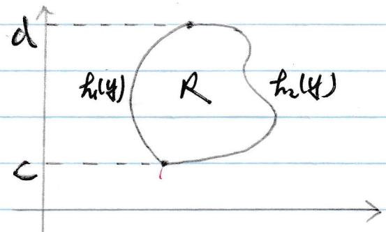
Then:  $\iint_R f(x, y) dA = \int_c^d \int_{h_1(y)}^{h_2(y)} f(x, y) dx dy$
