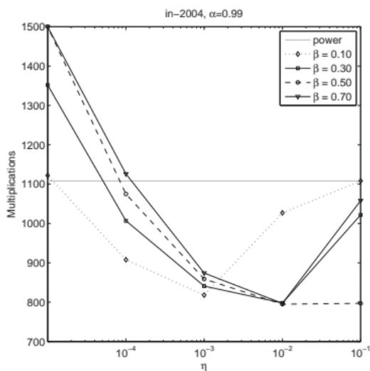
**Figure:** Total number of matrix-vector products required for convergence of the inner-outer scheme, for the in-2004 matrix. (Outer tolerance  $10^{-7}$ ,  $\alpha = 0.99$ ,  $\beta$ , and  $\eta$  varied. The iteration limit was 1500 and causes the ceiling on the left figure.)
