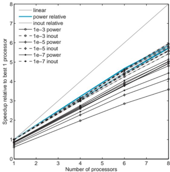
**Figure:** Parallel scalability for the three large graphs arabic-2005, sk-2005, and uk-2007. Light gray or teal lines are the relative speedup compared with the same algorithm on one processor. Black lines are the true speedup compared with the best single processor code. The parameters were  $\alpha = 0.99$ ,  $\beta = 0.5$ , and  $\eta = 10^{-2}$ .
