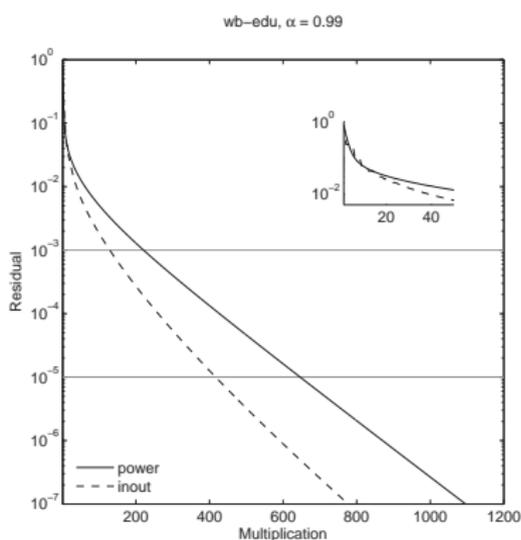
**Figure:** Convergence of the computation for the  $9,845,725 \times 9,845,725$  wb-edu matrix ( $\tau = 10^{-7}$ ,  $\beta = 0.5$  and  $\eta = 10^{-2}$  in the inner-outer method.) The interior figures highlight the first few iterations.
