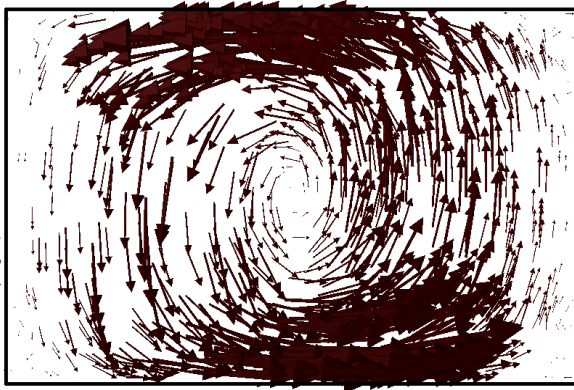
FIG. 7.4. Distribution of eddy current density on the cross-section of the lamination stack at x_1 = 0.0057 .
