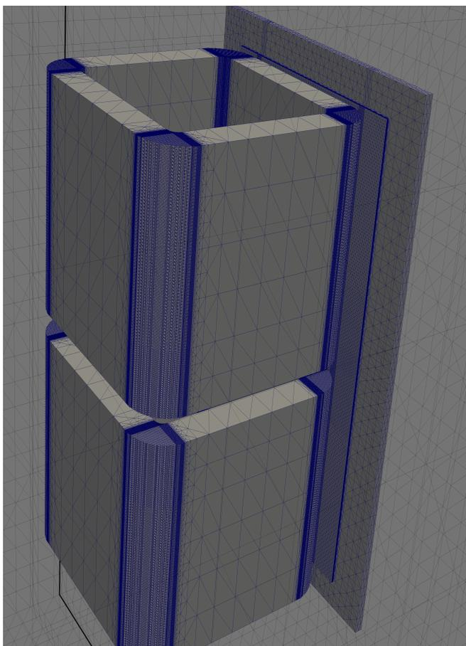
Fig. 6: Tetrahedral mesh of the coils and conductors.
