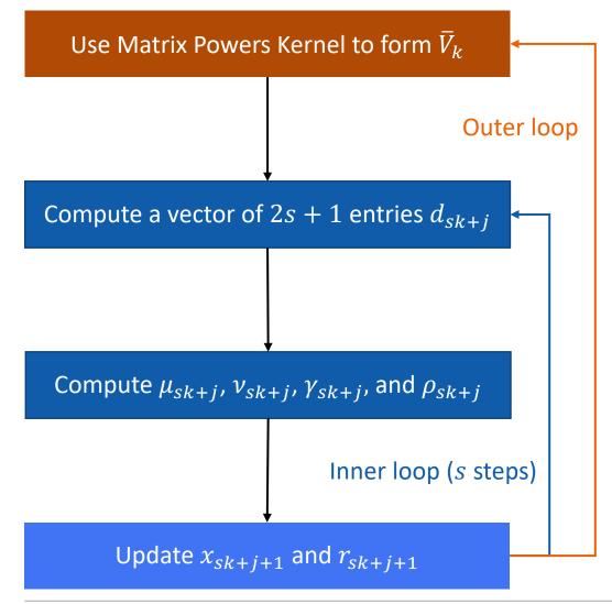
$$\begin{split} \bar{V}_k &:= \begin{bmatrix} v_{sk+1}, \dots, v_{sk+s} \end{bmatrix} \\ &\{v_{sk+i}\}_{i=1:s+1} = \operatorname{span}\{r_{sk+1}, Ar_{sk+1}, \dots, A^s r_{sk+1}\} \\ &\text{ is a basis of the Krylov subspace} \end{split}$$
