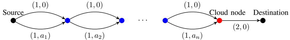
Fig. 1. The constructed network to prove Theorem 1(i), where the pair (c, d) over each link denotes that the communication capacity and the communication delay of the corresponding link are c and d , respectively.
