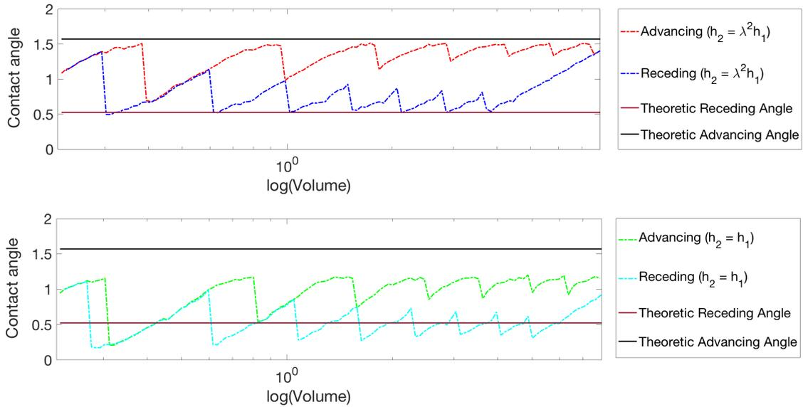
Figure 8: Advancing and receding contact angles for rough surfaces with  $\theta_Y = \pi/3$  and  $k = 10$  when  $h_2 = \lambda^2 h_1$  and  $h_2 = h_1$ , separately.
