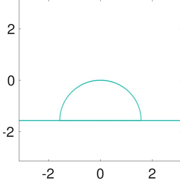
Figure 6: The half circle initial condition on the solid surface.
