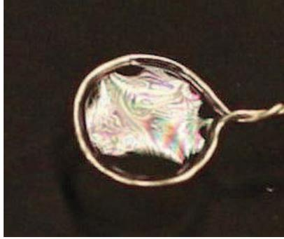
FIGURE 2. A metal ring of diameter 1 cm is used to support a soap film.
