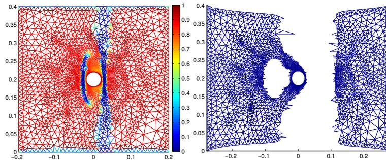
FIG. 8.5. *Uniaxial tension of a square with a rigid inclusion*,  $\lambda = 1.385$ ,  $\varepsilon = 0.001$ ,  $p = 3$ .
