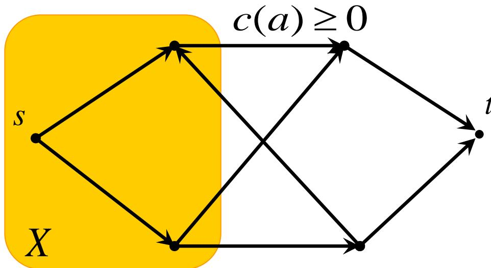
Max Flow Value = Min Cut Capacity
