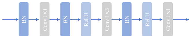
Fig. 2. Structure of dense layer. “Conv1 \times 3” denotes the convolutional layer with the kernel size 3 and the padding size (0,1).
