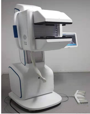
FIGURE 1. A prototype time-resolved diffuse optical tomography system designed for optical imaging of human breast [24]
